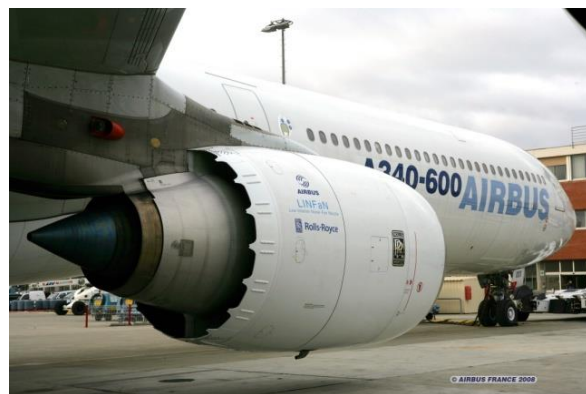
Figure 14: Low interior noise fan nozzle programme
