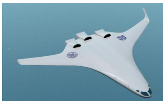
Figure 18: The 'Silent' Aircraft or blended-wing-body aircraft
